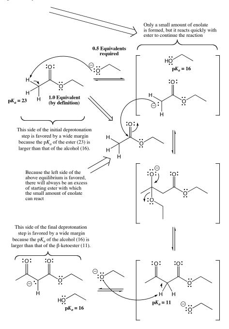
Because of this last step, one of these ethoxide molecules is consumed for every product molecule made. It takes 2 starting ester molecules to make a single product molecule, therefore, there is a two to one ratio of ester to base used. Because by definition 1.0 equivalent of ester is used in the reaction, the minimum amount of base required is 0.5 equivalents.
